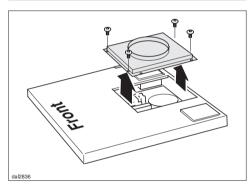
■ Remove the connection plate from the front of the appliance.
